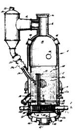
A coal supply gun assembly for a fluidized bed combustor which includes heat exchange elements extending above the bed's distributor plate assembly and in which the gun's nozzles are disposed relative to the heat exchange elements to only discharge granular coal material between adjacent heat exchange elements and in a path which is substantially equidistant from adjacent heat exchange elements.
